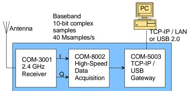
The samples can be read remotely over a TCP-IP link for further batch processing.
