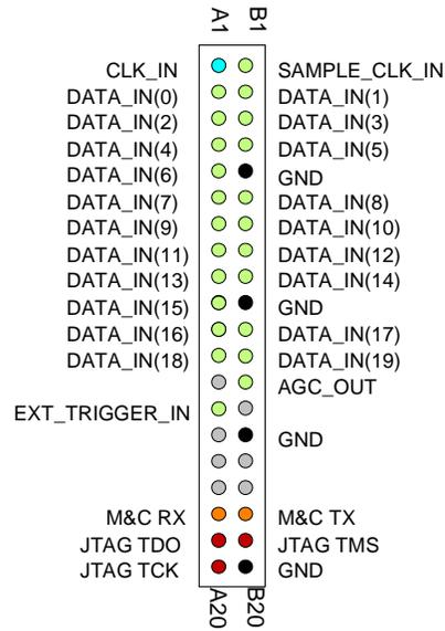
When input sample precision of less than 20 bits is selected, the lower ranking bits are used. For example, for a 2-bit precision input sample, DATA\_IN(0) and DATA\_IN(1) are used.
