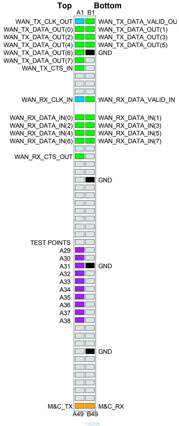
Configured as 8-bit parallel synchronous interface
