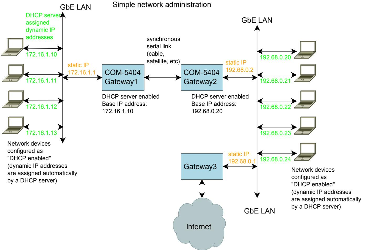
The diagram above illustrates a simple network administration scheme, whereby only gateways are administered with fixed (static) IP addresses. The other network devices automatically fetch their network configuration (IP address, subnet mask, DNS) from a DHCP server, like the one in the COM-5404.
