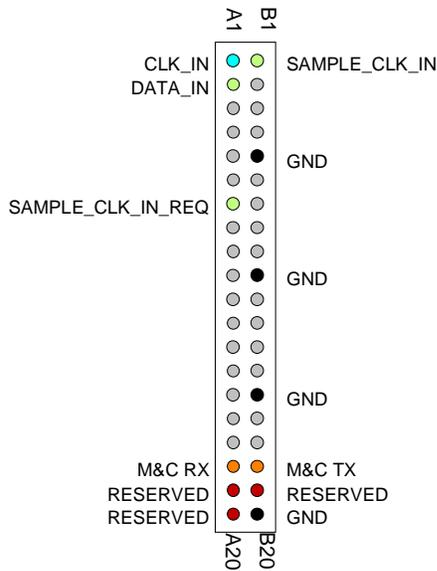
(b) 8-bit wide connection to another ComBlock [COM-5004, COM-8002, etc]
