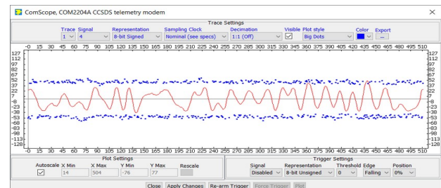
ComScope Window Sample: showing demodulated I symbols (blue), baseband input waveform (red)
