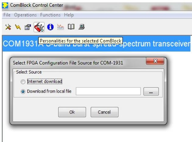
The software configuration files are named with the .bit extension. The bit file can be downloaded via the Internet, from the ComBlock CD or any other local file.
