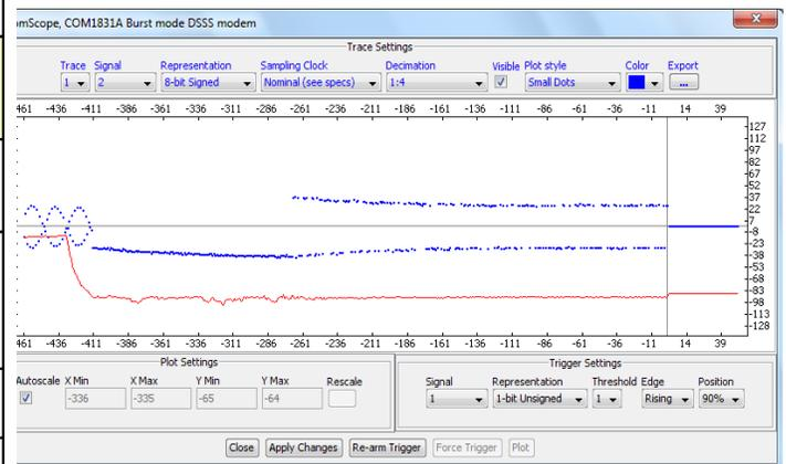
*ComScope example, showing trace1 signal2 (in blue): demodulated I-bits during preamble (left) then data (right half). Trace2 signal 4 (in red) shows the I-symbol tracking phase.*
