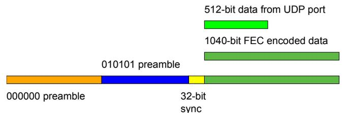
When transmitting multiple frames, follow-on frames are appended without preamble, separated only with a 32-bit sync word.
