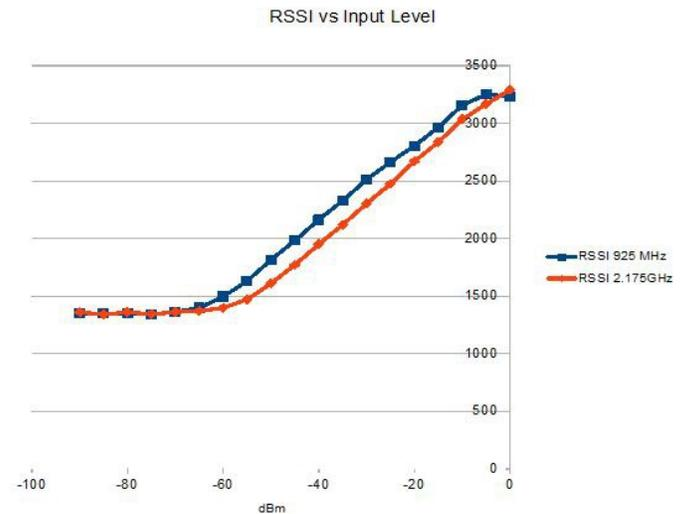
Note: RSSI measurement below -50Bm is affected by the presence of 10 MHz frequency reference when supplied to an external LNB (see control register REG46(2)).
