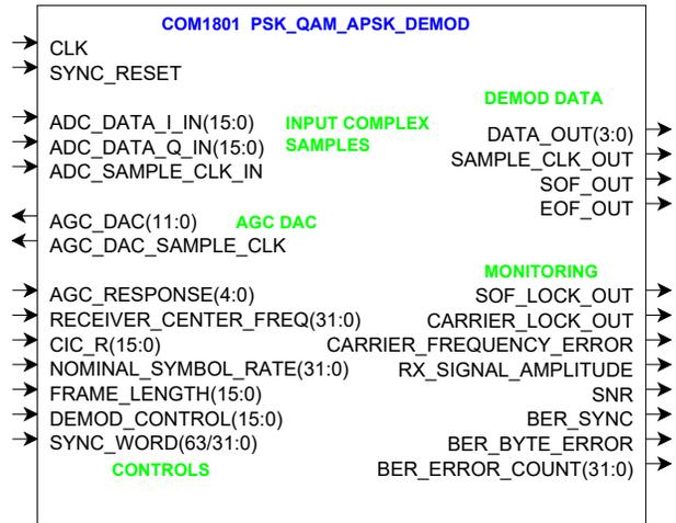
**ADC\_DATA\_I/Q\_IN(15:0)**: input samples from one or two external ADCs. (one in the case of IF undersampling, two for near-zero frequency complex inputs). If the ADCs have fewer than 16-bit precision, align the most significant bit with ADC\_DATA\_IN(15). Format: 2's complement (signed).
