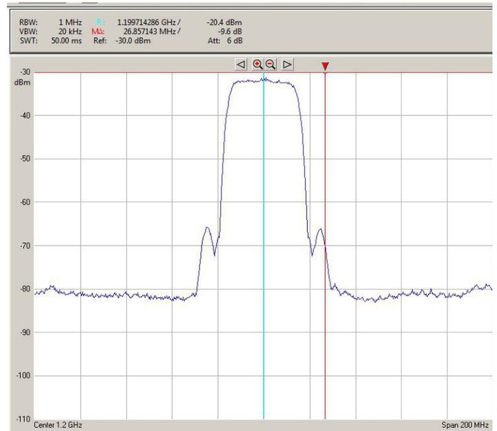
Output spectrum (after D/A conversion and RF modulation): 30 Mchips/s
