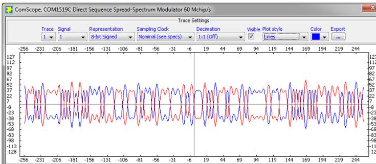
ComScope Window Sample: showing the modulated output waveform: blue for I-channel, red for Q-channel.
