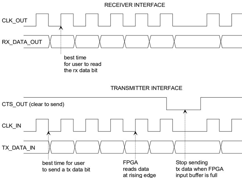
In the transmit direction, the user provides both clock (CLK\_IN) and data (TX\_DATA\_IN). The user should always check the “Clear-To-Send” CTS\_OUT flag before sending additional data bits to the modulator. As option **-B** includes HDLC, the user is allowed not to transmit data. When so, the modem will send empty HDLC frames.
