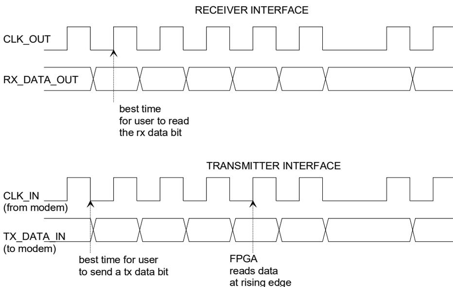
In the transmit direction, the user provides serial data (TX\_DATA\_IN), preferably at the falling edge of the modem-supplied CLK\_IN. The TX\_DATA\_IN is read at the rising edge of CLK\_IN. The user **MUST** provide data, otherwise an underflow condition will occur. Option **-C** is for continuous-mode operation. No gap in data
