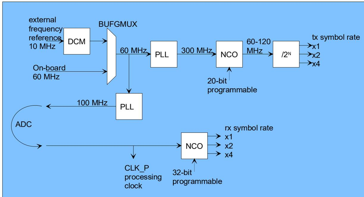
The software is written to accept a 10 MHz or a 60 MHz clock as frequency reference.
