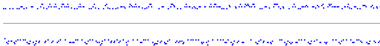
ComScope Window Sample: showing the demodulated symbols at the symbol center (blue trace1/signal 2, dots)
