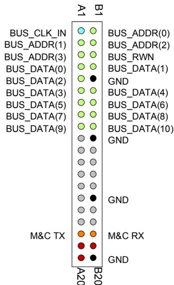
This connector is used for multipoint-to-point connection over a shared data bus when control register REG8(4) = '1'. COM-1027 is a bus slave. It always listens to BUS\_CLK\_IN, BUS\_ADDR, BUS\_RWN.
