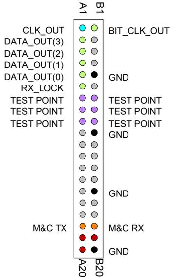
This connector is used for point-to-point (i.e. direct) connection between two ComBlocks when control register REG8(4) = '0'.
