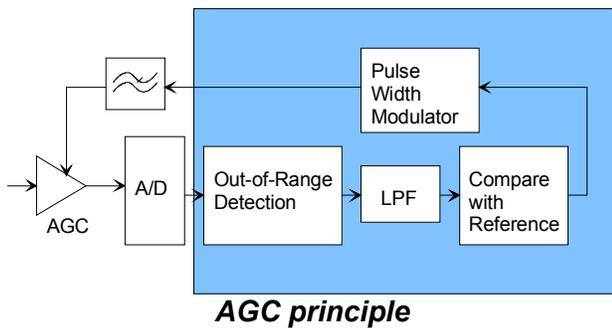
The analog circuit shall filter this 3.3V low-voltage TTL PWM signal with a low-pass filter prior to controlling the analog gain. The PWM is randomized and its spectral distribution shifted to the higher frequencies so as facilitate the analog low-pass filter design.
