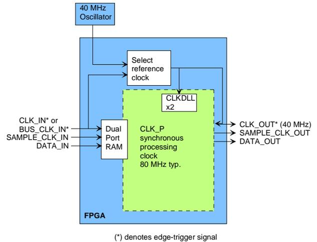
When the internal reference clock is selected, the processing clock  $f_{clk}$  is not related to the CLK\_IN clock frequency. In this case, the role of CLK\_IN is restricted to that of input clock. It can therefore take any frequency value up to the maximum of 40 MHz.
