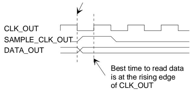
Point to Multi-points connection (REG19 bit4 = 1). COM-1019 is a bus slave. It always listens to BUS\_CLK\_IN, BUS\_ADDR, BUS\_RWn.
