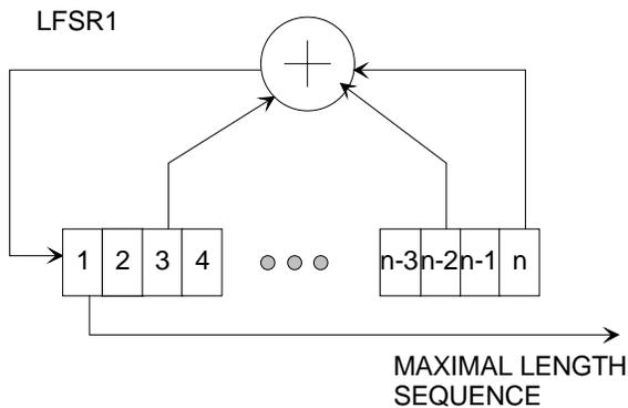
The code period is  $2^n - 1$ , where n is the number of taps in the shift register. The LFSRs are initialized to all 1's at the start of each period. The LFSRs will generate all possible n-bit combinations, except the all zeros combination.
