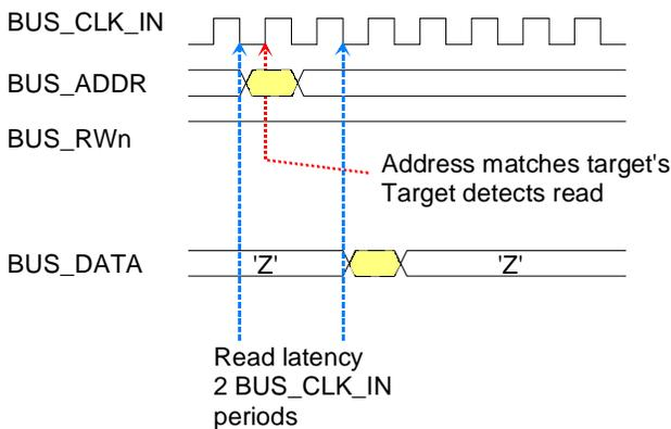
Master reads flow control from COM-1019 target
