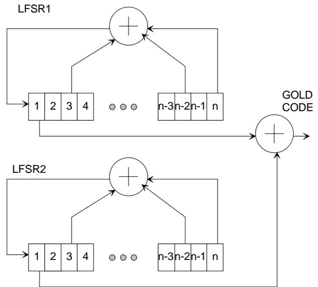
The code period is  $2^n - 1$ , where n is the number of taps in the shift register. The LFSRs are initialized to all 1's at the start of each period. The LFSRs will generate all possible n-bit combinations, except the all zeros combination.
