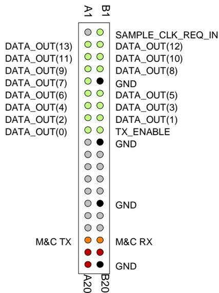
This connector is used when output data is pulled out by the next module (configuration REG19 bit 0 = 1).
