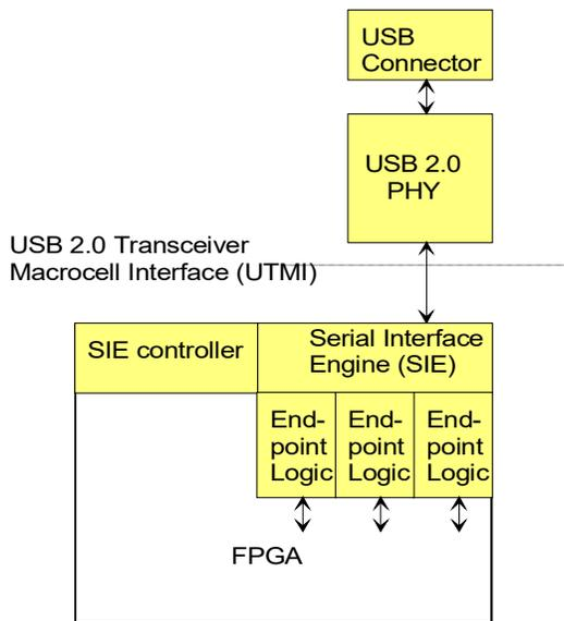
The interface between the FPGA and the USB 2.0 PHY transceiver is a standard as described by the “USB 2.0 Transceiver Macrocell Interface (UTMI) Specifications”, Version 1.05 3/29/2001 found at [www.usb.org](http://www.usb.org)
