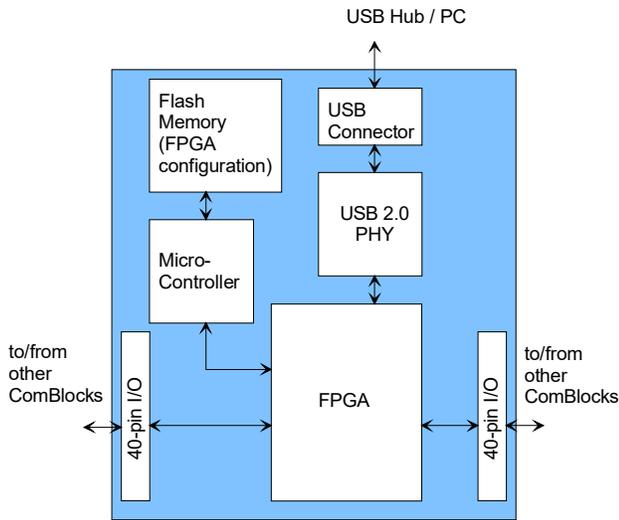
**Block Diagram of ComBlock as USB 2.0 Device**
