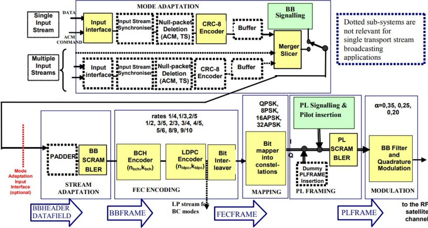
Figure 1: Functional block diagram of the DVB-S2 System
